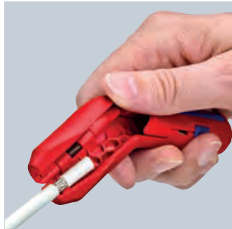
Stripping of a coax cable
